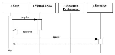
The virtual proxy, obtained from e.g. a Factory [GHJV95] by the user, intercepts the acquisition request and returns an eagerly acquired resource. The resource user can now access and use the resource.
