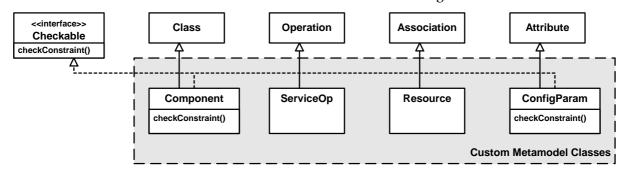
When the parser analyzes the model (it is represented as an XMI file) it instantiates the metamodel classes based on the stereotypes. The metaclasses shown above can contain custom functionality such as constraint checking. We provide the interface *Checkable* in the metamodel. The following shows the code that needs to be implemented to ensure that *ConfigParams* can only be attributes of type *String*.
