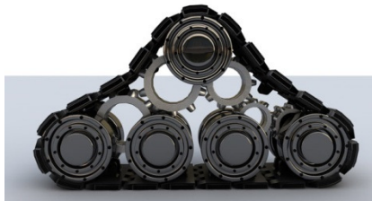
Fig 12. Triangular driver and follower wheels arrangement
