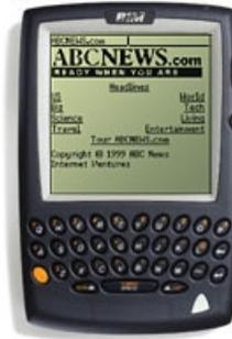
**Figure 2: Browsing the Web on a wireless PDA with 512 KBytes of SRAM.**
