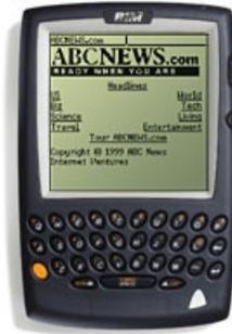
**Figure 2: Browsing the Web on a wireless PDA with 512 KBytes of SRAM.**
