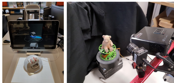
Fig. 4. Automatic 3D scan with HP sprout, and DIY camera setup for 3D scan.
