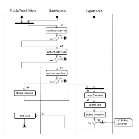
Figure 2 Activity Diagram for Use Case Drop Off Export Container
