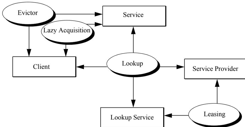
The picture shows that the Evictor pattern is used by clients to evict services. The Lazy Acquisition pattern is used during the client's acquisition of a service. The Lookup pattern is used first by a service provider to register a service with the lookup service, and then by a client to look up a service from the lookup service. Finally, the Leasing pattern is used by the service provider for registrations at the lookup service.
