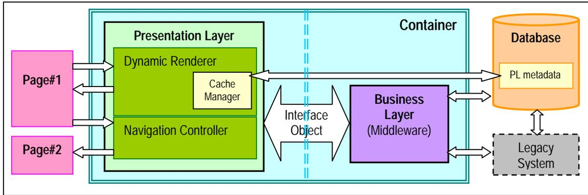
Figure 2: Architecturally significant elements of an enterprise Web system
