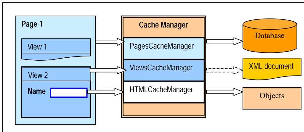
Figure 18: Example of cache manager to cache data from several sources
