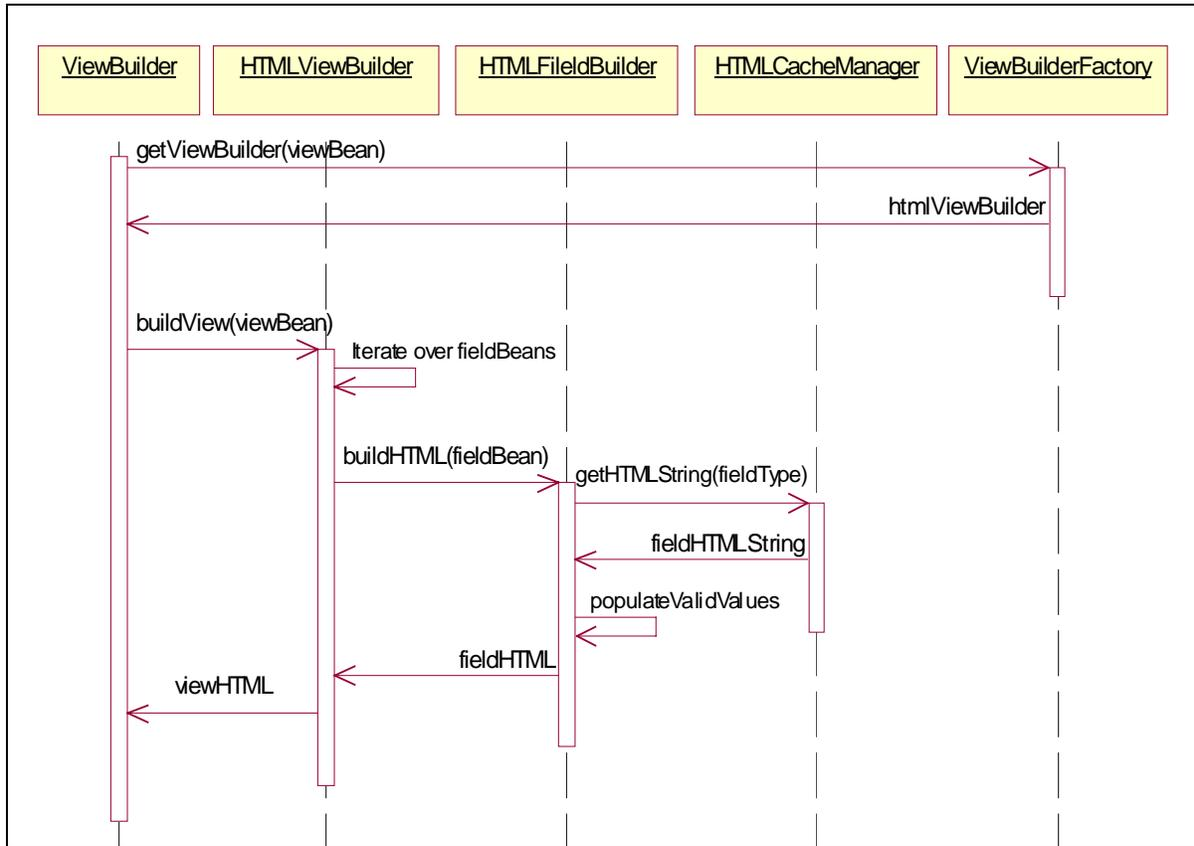
Figure 16: Sequence diagram for generating view HTML
