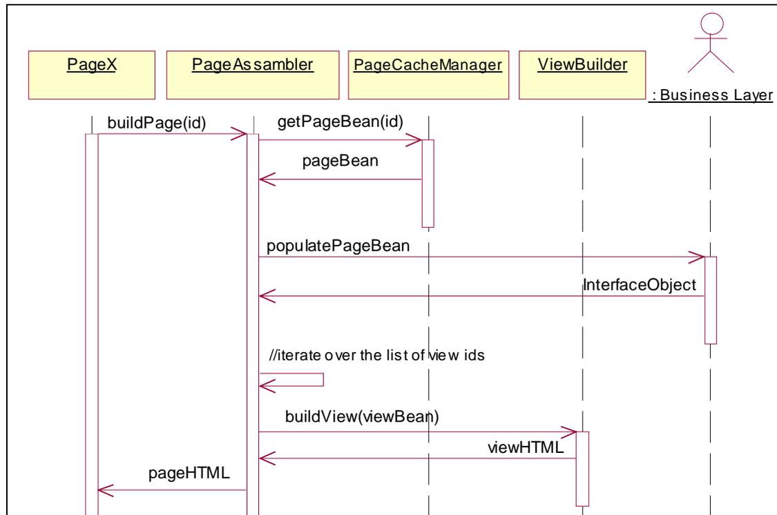
Figure 13: dynamic page assembling sequence diagram
