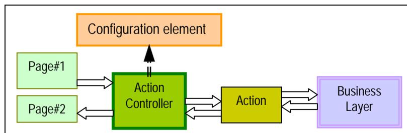
Figure 5: A typical navigation controller structure
