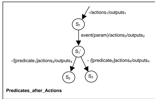
**Figure 3. State Transition Diagram of CEFMSM with Predicates after Actions**
