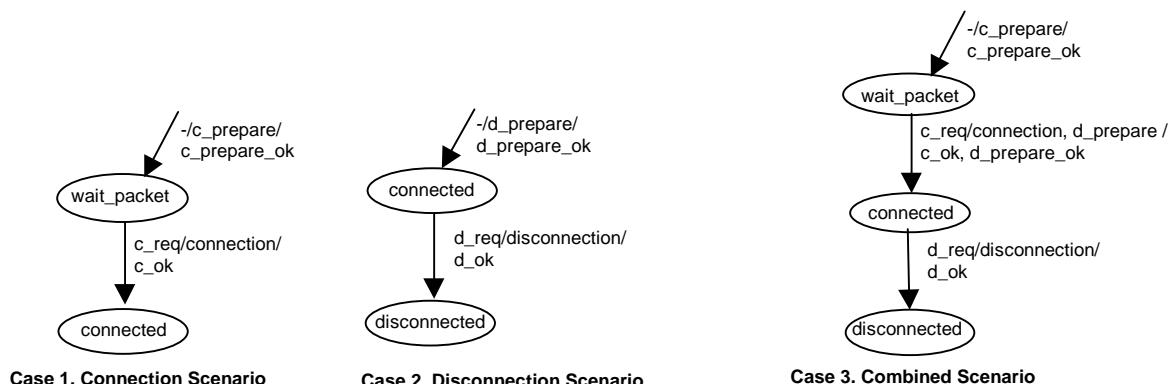
Figure 20. Packet Handling CEFMS using Sequential Merge
