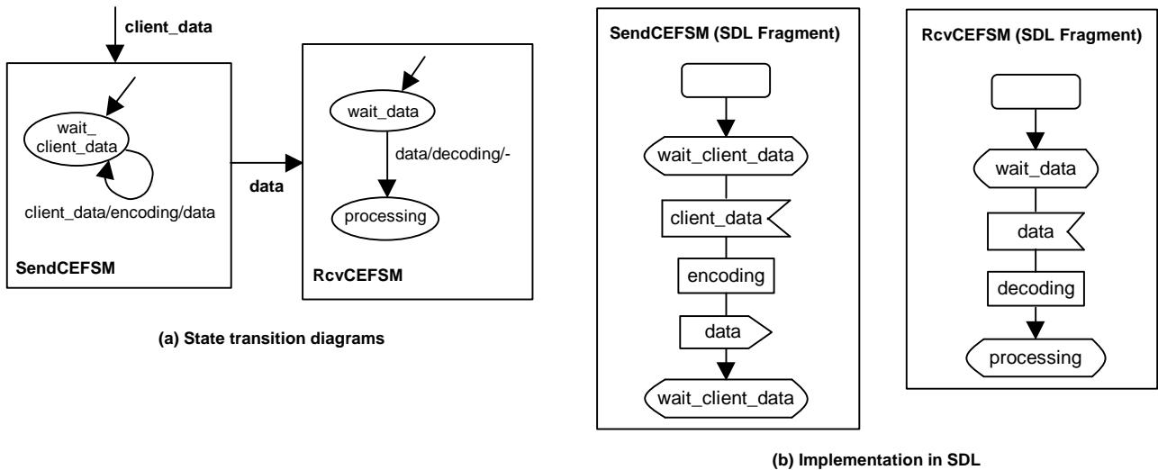
Figure 9. Simple Data Transfer Using Basic CEFMSMs
