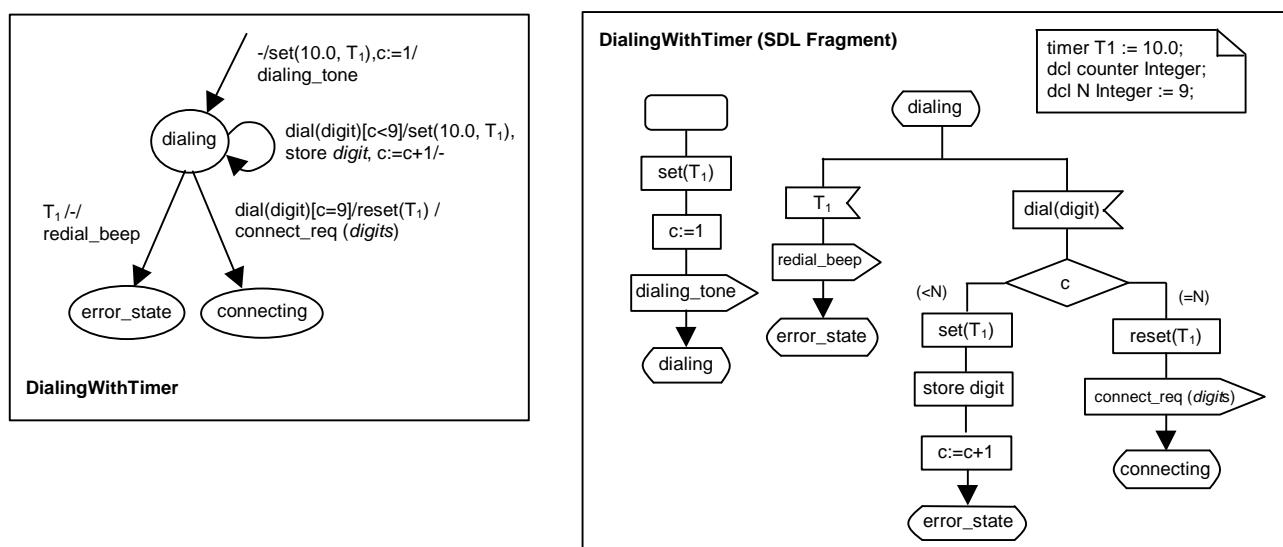
Figure 24. Nine Digit Dialing with a Timing Constraint
