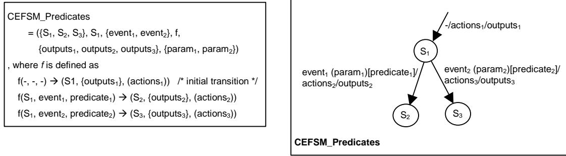
**Figure 2. CEFMSM with Predicates and its State Transition Diagram**
