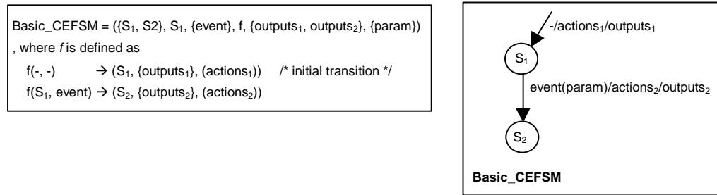
Figure 1. Basic CEFMSM and its State Transition Diagram
