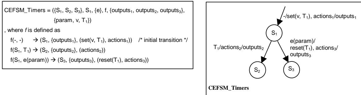
Figure 4. CEFSM with Timers and its State Transition Diagram
