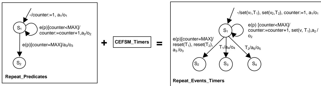
Figure 22. Handling Repeated Events with Timers
