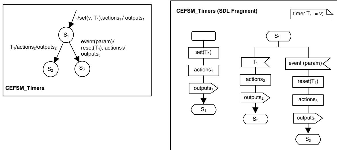
Figure 8. Translation of CEFSM with timers into SDL
