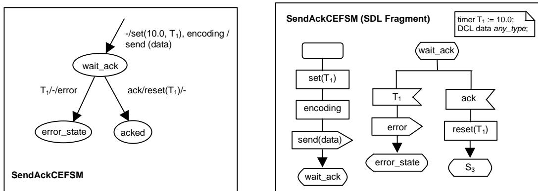
Figure 12. Example of Confirmed Data Transfer with a Timer
