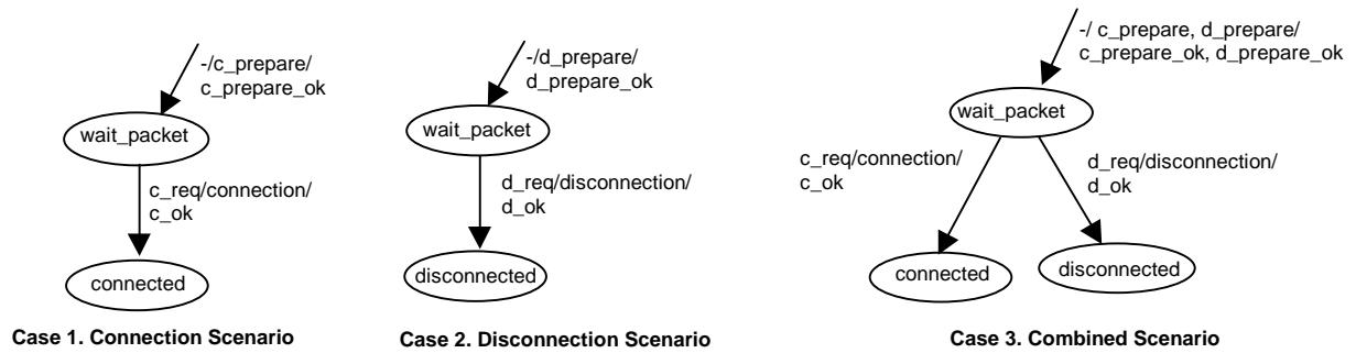
Figure 19. Packet Handling CEFMS using Source Merge
