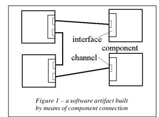
Components that just provide services are not the general case in componentoriented development. If an application is built only with components, as shown in figure 1, one component will require the services from other components. So, it is not reasonable a component description including only provided services. Required services need to be specified too. So, in general case, component interaction is bidirectional [OLA 96].
