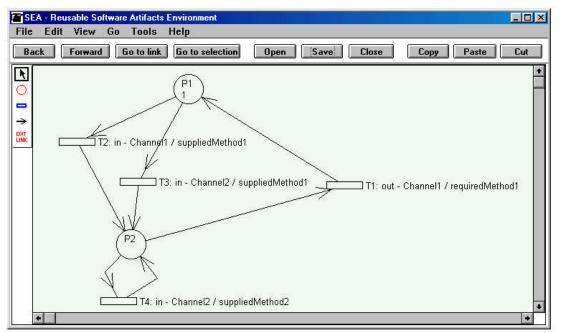
Figure 3 – Behavioral specification of a component interface based on Petri net
