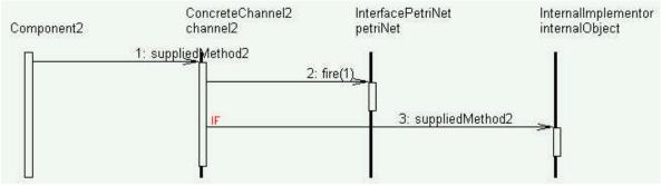
Figure 9 – A component receiving a method requirement from another component
