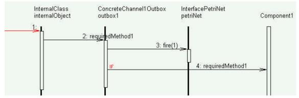
Figure 8 – A component sending a method requirement to another component
