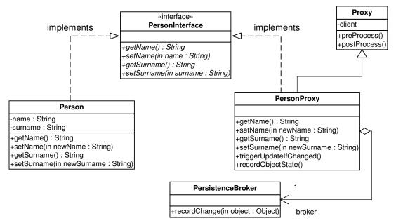
As in the second variation, the interface PersonInterface is used to connect the application layer (class Person) with the interception layer (abstract class Proxy and concrete class PersonProxy). The class PersistenceBroker is part of the framework layer.
