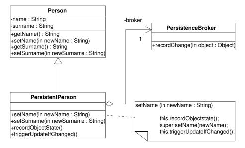
In this pattern the class Person would be part of the application layer, the class PersistenceBroker would be part of the framework layer and the class PersistentPerson (which makes the connection between them) would be part of the interception layer.
