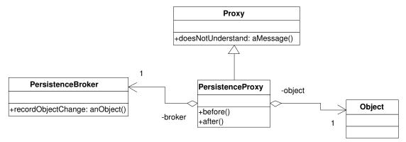
In this pattern the classes Proxy and PersistenceProxy would be placed in the interception layer, the class PersistenceBroker would be placed in the framework layer and the proxy's subject in the application layer.
