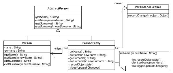
In this variation the class AbstractPerson is used to establish class-based constraints. The class Person is part of the application layer, the class PersonProxy is part of the interception layer and the class PersistenceBroker is part of the framework layer.
