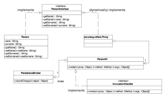
In this variation the interface PersonInterface is the key to connect the application layer (class Person) with the interception layer (class Proxy); the broker is part of the framework layer.
