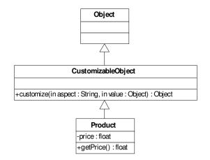
As we can see in the figure, the class Product is a subclass of CustomizableObject instead of Object. If we think in terms of a three layered architecture, the class CustomizableObject would be in the interception layer and the class Product in the domain layer.
