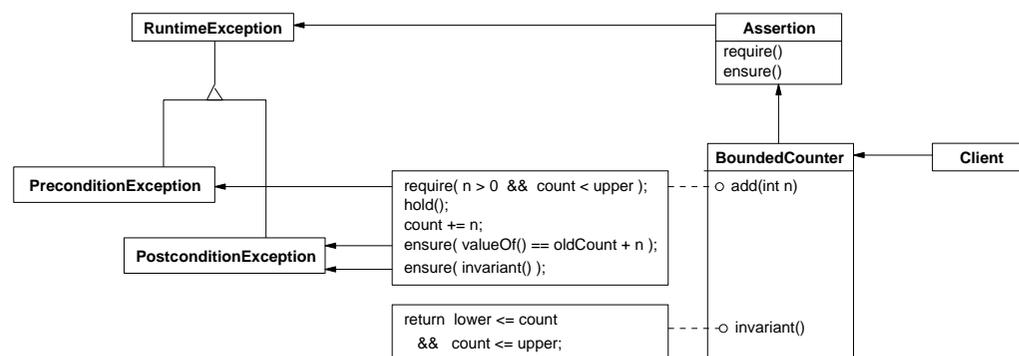
This diagram illustrates how the *Contract* pattern offers a solution. The implementation of the bounded counter is robust, since it guards clients against possible misuse. The advantage of using assertions, apart from providing checks to legal usage, is that they explicitly state the requirements imposed on the client and on the supplier.
