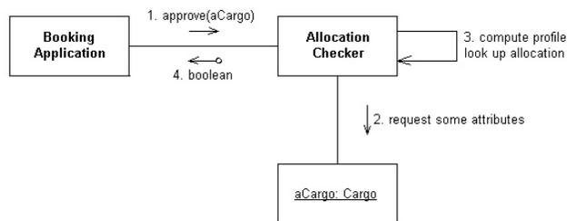
The only remaining issue is the translation between the two contexts. In this case, the only information that is being exchanged is (as modeled in our context) the **Allocation** and the **Cargo Profile**. Translations must be defined between these and the equivalent representations in the alien tool.
