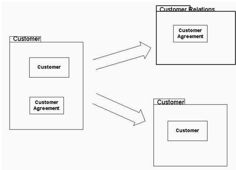
I hate introducing new notation, but I know of no way of laying emphasis on some packages over others in UML, so I have drawn the core domain packages in a bolder line. In laying out diagrams of many packages, I attempt to convey the importance of those packages subjectively by placing them centrally, but this is only an aide and some notational distinction is needed to be unambiguous.
