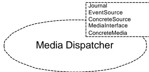
Figure 15: The Parameterized Collaboration representation for Media Dispatcher Pattern
