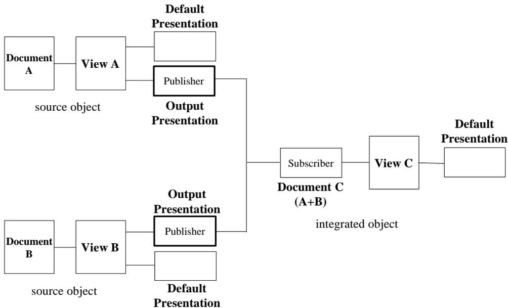
Fig. 4 An integrated object could be easily obtained by attaching an additional *output presentation* to each source object.
