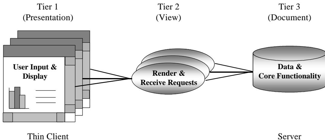
Fig. 7 The DVP pattern divides an interactive application into three tiers.
