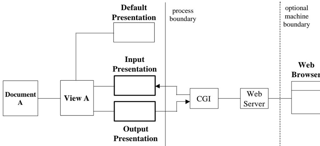
Fig. 5. Discover could be controlled by a Web browser through the cooperation between the *input presentation* and the *output presentation*.
