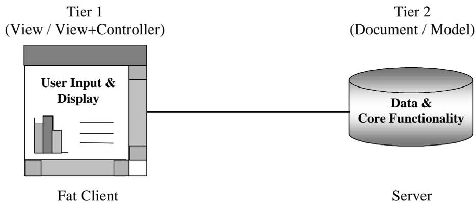
Fig. 6. Both MVC and DV patterns divide an interactive application into two tiers.
