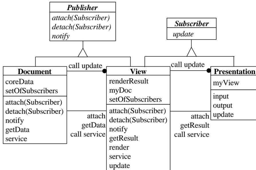
Fig. 3 The object model of DVP with Object Modeling Technique (OMT)<sup>6</sup> notation.
