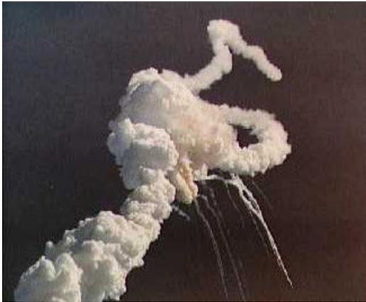
On January 28, 1986 the space shuttle Challenger exploded. The cause was in part determined to be due to a hurried cold weather launch and a subsequent seal failure in the solid rocket booster. O-Rings do not seal properly in cold weather, even when commanded to by politicians.<sup>12</sup>
