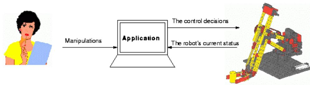
Figure 1. A Computer-supported Robot Control System
